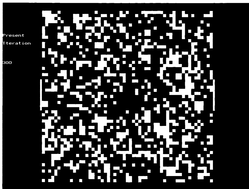
Fig. 3. Configuration of parameter set 14 after 300 iterations showing the direct diffusion of unbound solute cells away from the solute block.
